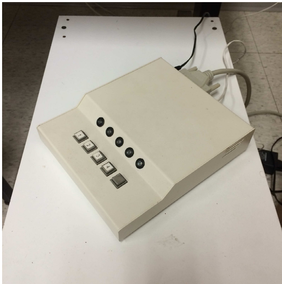
Figure 6. Detailed picture of the serial response box.
