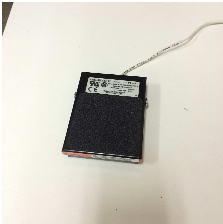
Figure 16. Detailed picture of the footswitch.
